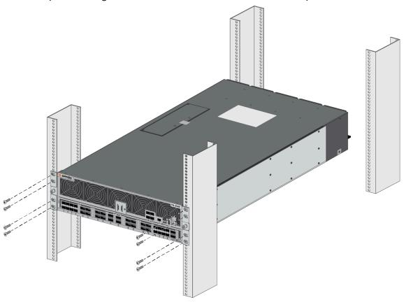
STEP 3 | Slide one adjustable rack mount bracket into each of the two previously installed fixed rack mount bracket. Secure the two adjustable rack mount brackets to the back rack-posts using
