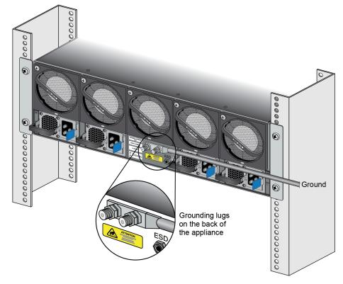
STEP 5 | Crimp a 6-AWG wire to the provided grounding lug and connect the other end to your earth ground point.
