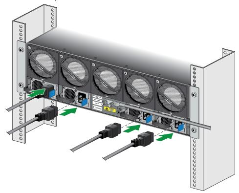
2. Secure the power cords to the power inlets using the velcro straps.
