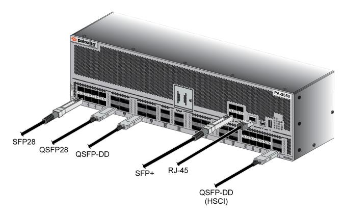
The next image shows the PA-5560, PA-5570, and PA-5580 firewall cable connections.
