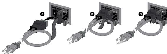
**STEP 5 |** Connect the other end of the power cords to an AC power source. After the first power supply is connected, the firewall powers on and the power LED on the power supply and the PWR LED on the front of the firewall turns green.
