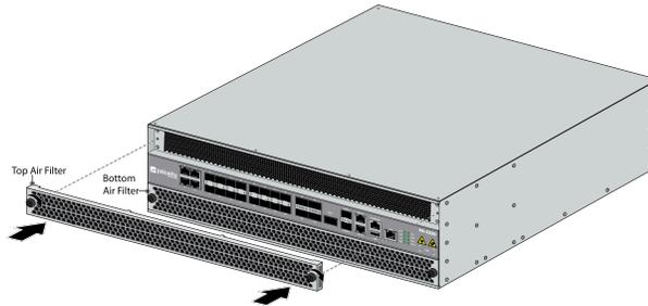
**STEP 5 |** Repeat this procedure to replace the bottom air filter.
