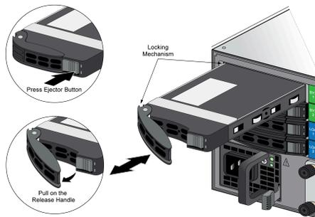
**STEP 5 |** Remove the replacement drive from the packaging, determine the drive model, and place it on an antistatic surface. Then compare this model number with the model number of the failed drive to determine which replacement procedure to use in 7.
