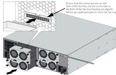
**STEP 4 |** Slide the replacement fan tray into the empty fan-tray slot ensuring that the alignment grooves on the fan tray and the fan-tray slot are aligned. Push the tray in until it seats and then turn the four fan-tray thumb screws clockwise to secure the tray to the firewall.
