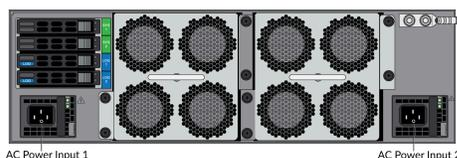
**STEP 4 |** Secure the power cords to the power supplies using the Velcro straps.
