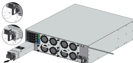
**STEP 5 |** Remove the replacement power supply from the packaging and slide it into the empty power supply slot. Push the power supply all the way in until the release lever clicks and secures the power supply.
