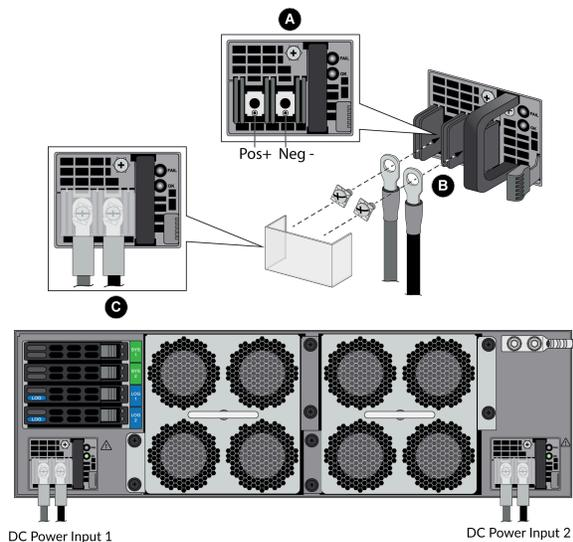
**STEP 5 |** After all DC power cables are securely connected, power on the DC power source.
