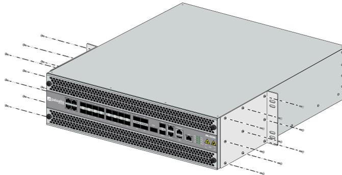
**STEP 2 |** With help from two other people, hold the firewall in place in the rack and secure the rack-mount brackets to the rack using four screws for each bracket. Use the appropriate screws (#10-32 x 3/4" or #12-24 x 1/2") for your rack and torque to 25 in-lbs. Use cage nuts (not provided) to secure the screws if the rack has square holes.
