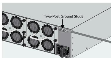
**STEP 2 |** Crimp a 6AWG ground cable (not included) to the two-hole 6AWG ground lug and then attach the ground lug to the ground studs on the firewall. Replace the star washers and nuts and torque to 25 in-lbs. Connect the other end of the cable to earth ground.
