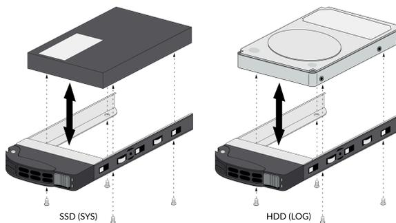
**STEP 6 |** Install the carrier with the replacement drive:
