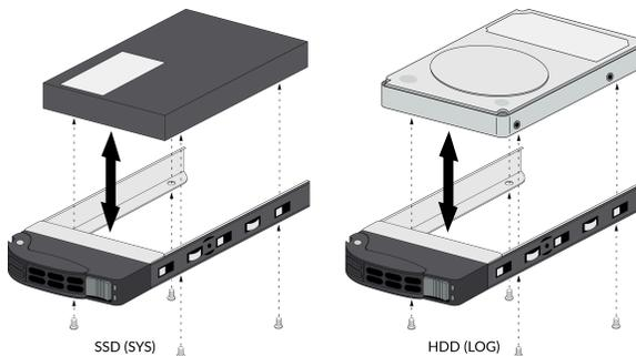
**STEP 7 |** Install the replacement drive in the firewall.
