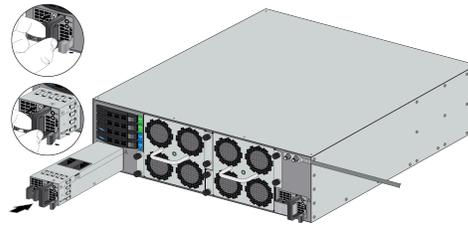
**STEP 6 |** Reconnect the positive and negative DC power cables to the new power supply using the DC terminal screws.
