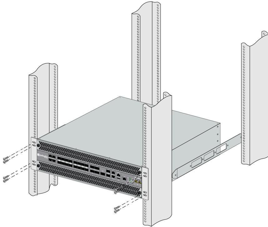
**STEP 4 |** Slide one back rack-mount bracket onto each of the two previously installed side rack-mount rails and secure the brackets to the back rack posts using four screws for each bracket (#10-32 x 3/4" or #12-24 x 1/2") and torque to 25 in-lbs. Use cage nuts (not provided) to secure the screws if the rack has square holes.
