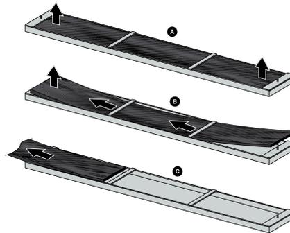
**STEP 3 |** Install a new filter into the filter cover ensuring that you slide it under the filter cover cross bars. You can install the filter with either side facing up.
