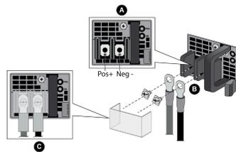
**STEP 7 |** When all DC power cables are securely connected and the plastic guard is properly reattached, power on the DC power source.
