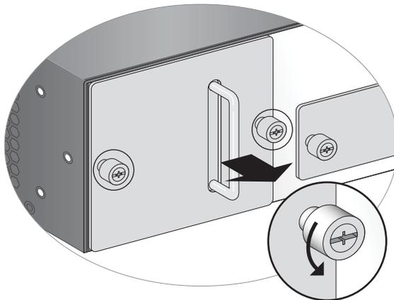
**Figure 17. Loosening the Thumbnail Screws for the Fan Tray and Air Filter**
