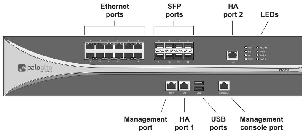
**Figure 2. PA-5020 Front Panel**
