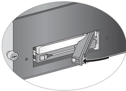
**Figure 16. Replacing a Drive**
