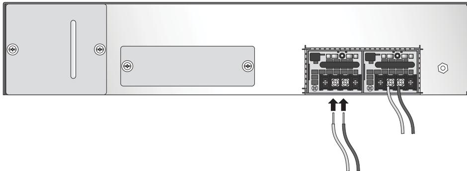
**Figure 8. DC Power Supply - Attachment**
