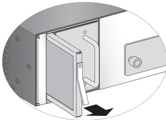
**Figure 19. Removing the Air Filter**
