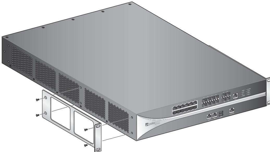
**Figure 4. Attaching Rack Mounting Brackets**
