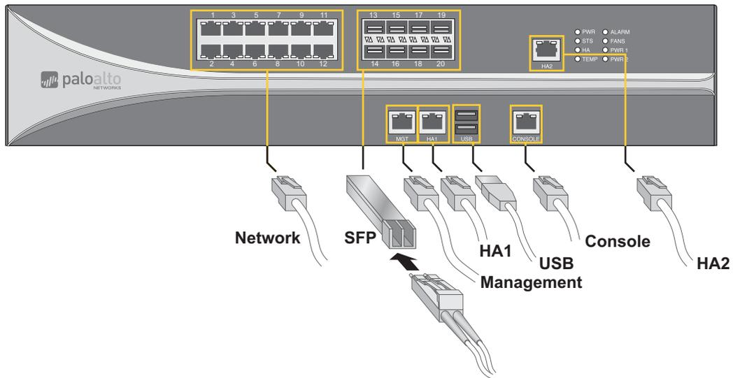
**Figure 6. Cable Connections for the PA-5020**
