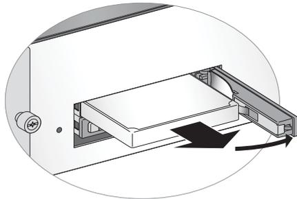
**Figure 15. Removing a Drive**
