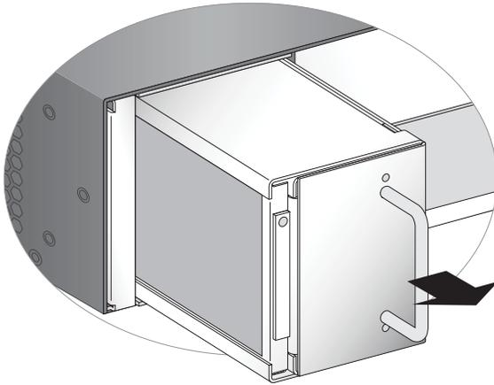
**Figure 18. Removing the Fan Tray and Air Filter**
