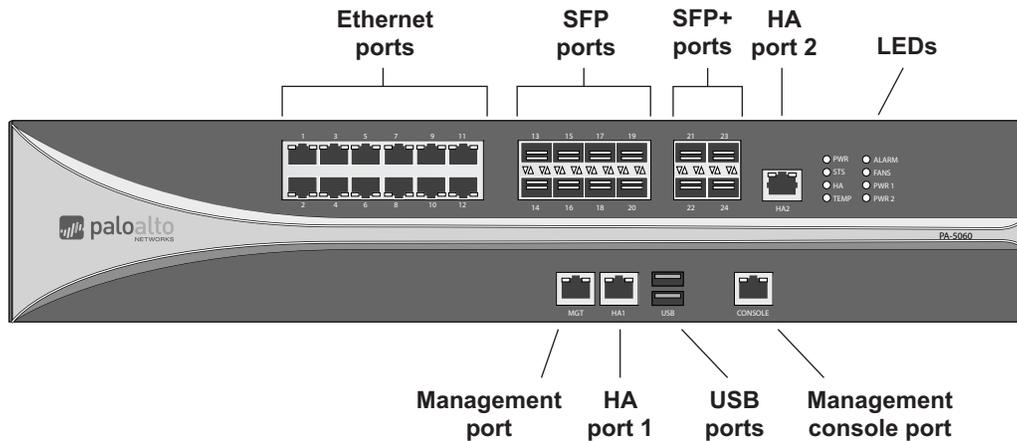
**Figure 1. PA-5060 and PA-5050 Front Panel**
