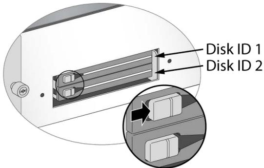
**Figure 14. Releasing a Drive**
