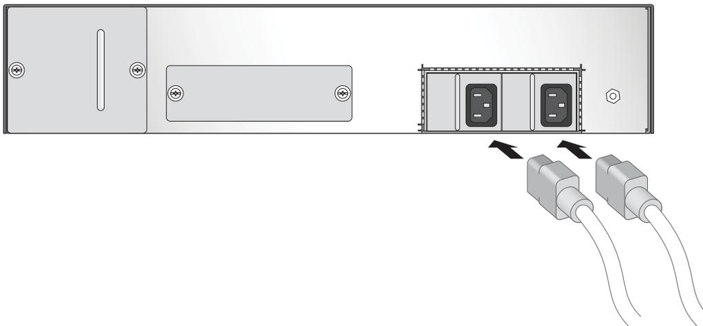
**Figure 7. Power Connection for the PA-5000 Series**
