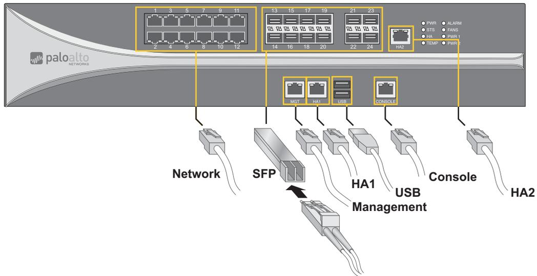
**Figure 5. Cable Connections for the PA-5060 and PA-5050**
