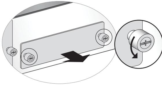
**Figure 13. Loosening the Thumbnail Screws for the Drive Bay**
