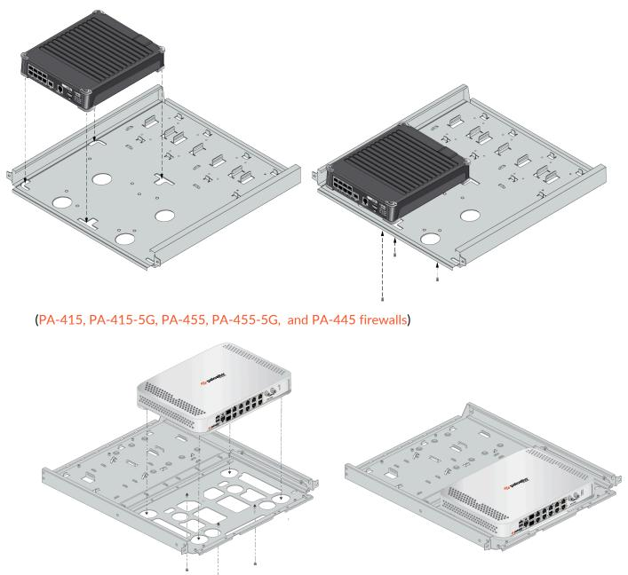
**STEP 5** While holding the firewall, carefully flip the mounting tray over to reveal its underside.
