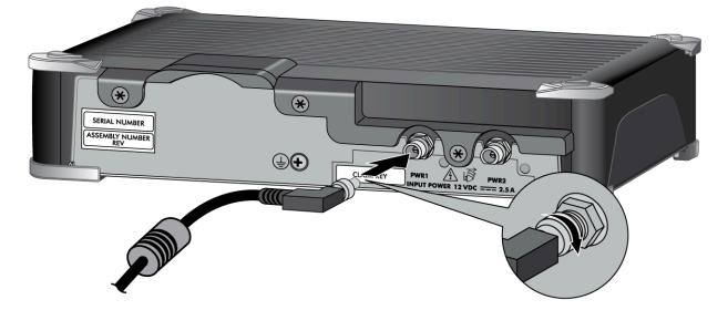
**STEP 4** | Plug the connector from the power adapter into your power source. After power is connected, the firewall powers on as indicated by the green power LED next to the PWR 1 port. The front PWR LED shows green when a functioning power adapter is connected.
