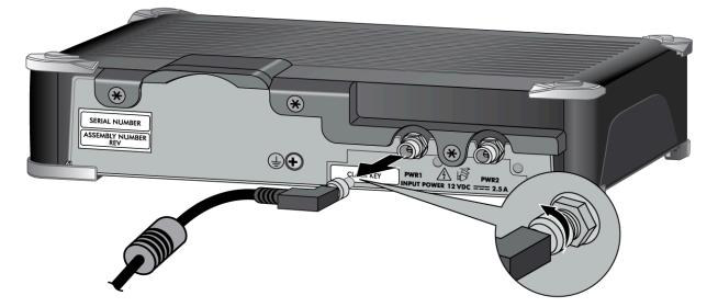
(PA-410) Unplug the failed power adapter from the AC power source and pull the power cable out of the firewall to remove it.
