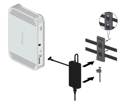
**STEP 5** After you secure the power adapter to the bracket, mount the bracket next to the firewall using wood or drywall screws as appropriate.
