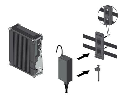
(PA-415, PA-415-5G, PA-455, PA-455-5G, and PA-445) Install the power adapter in the power adapter wall-mount bracket using the Velcro straps and cable tie. Make sure to align the cable tie with the notches in the bracket to prevent the power cord from falling out. Next, loop the two Velcro straps through the side openings on the wall mount and over the power
