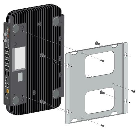
**STEP 4** Install the power adapter in the power adapter wall-mount bracket.
