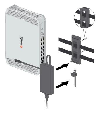
(PA-410) Install the power adapter in the power adapter wall-mount bracket using the Velcro straps and cable tie. Make sure to align the cable tie with the notches in the bracket to prevent the power cord from falling out. Next, loop the two Velcro straps through the side openings on
