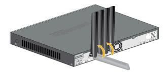
**STEP 2** Adjust the antenna orientation to receive the optimal signal strength in your environment.
