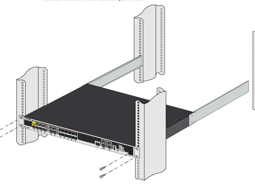
STEP 4 | Slide one back rack-mount bracket into each of the two previously installed side rack-mount rails and secure the brackets to the back rack-posts using the appropriate screws for your rack (#10-32 x 3/4" or #12-24 x 1/2") and torque to 25 in-lbs.
