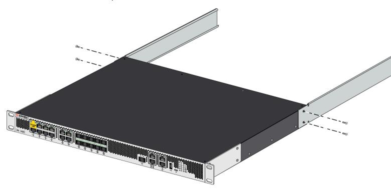
STEP 3 | With help from another person, hold the firewall in the rack and secure the front rack-mount brackets to the front rack-posts using two screws for each bracket. Use the appropriate
