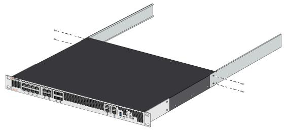
**STEP 3** Hold the device in the rack and secure the front rack-mount brackets to the front rack-posts using two screws for each bracket. Use the appropriate screws (#10-32 x 3/4" or #12-24 x
