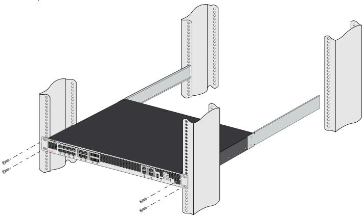
1/2") for your rack and torque to 25 in-lbs. Use cage nuts to secure the screws if the rack has square holes.
