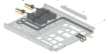
STEP 6 | Plug the power supply connector into the back of the device. Using the provided tie-wraps, bind and secure the power supply cable toward the back end of the tray using the sheet-metal lances toward the center of the tray.
