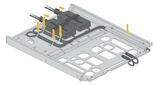
STEP 7 | With the front of the device facing forward, align the four rubber feet on the bottom of the device to the slotted holes in the provided mounting tray. Secure the device in place using two provided #6-32 x 3/16" Long Flathead screws.
