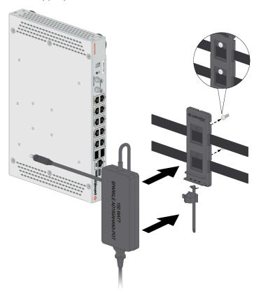
The following image shows a completed installation for an ION 3200 with a single power adapter.
