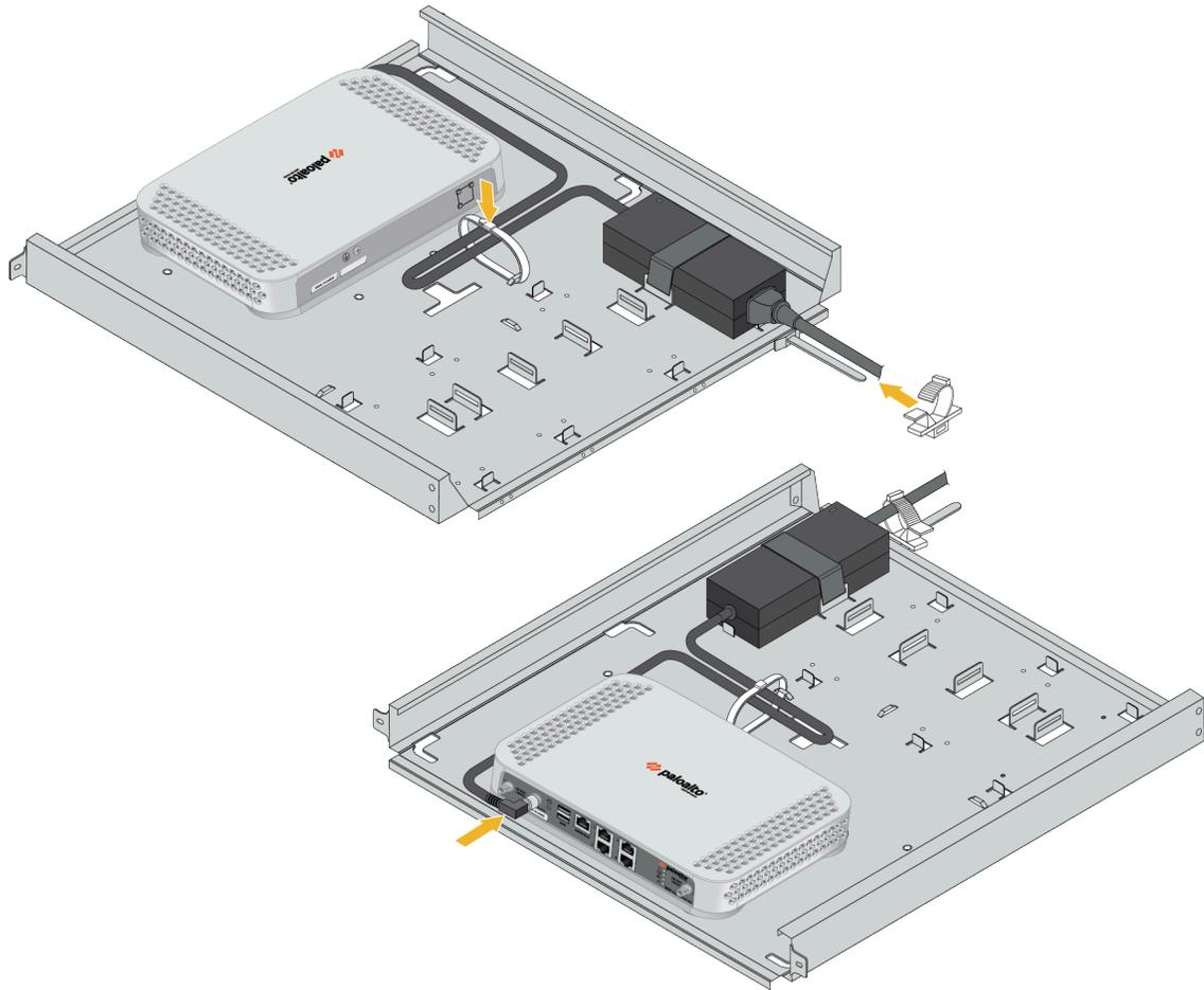
**STEP 8 |** Slide the mounting tray into the rails previously fixed to the equipment rack. Stop when the front flange on the mounting tray is flush with the front of the rail.
