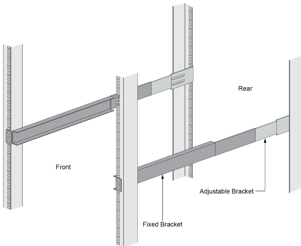
**STEP 2 |** Align the bottom edge of the mounting rails to the bottom of the 1 RU rack space reserved for the device. Align the slotted holes in the adjustable mounting bracket to the holes on the rear of the equipment frame.
