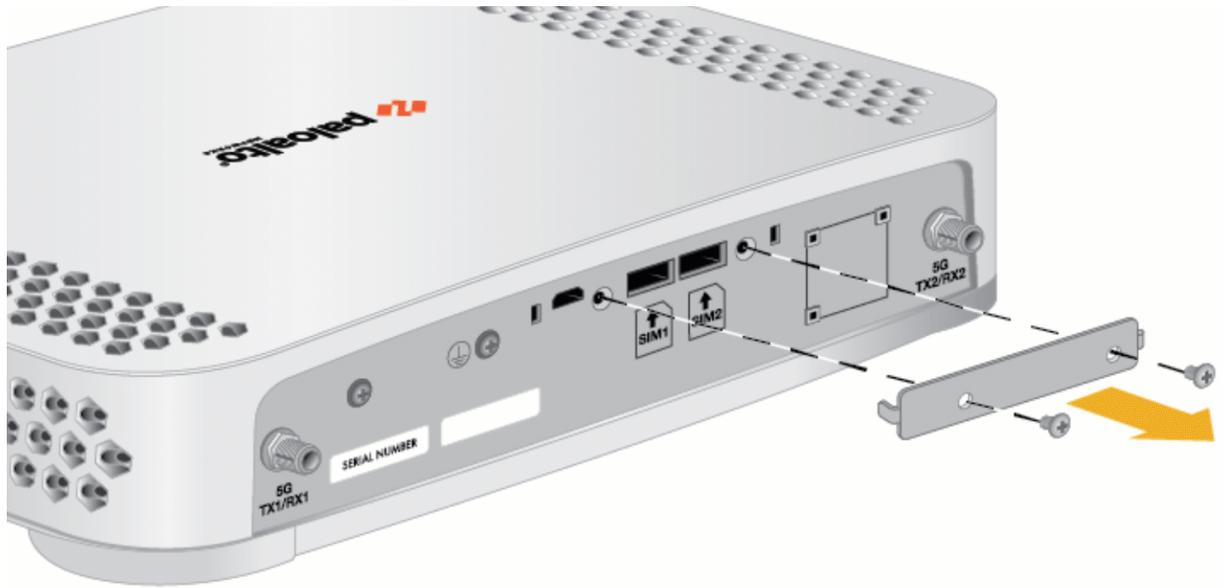
**STEP 3 |** After inserting the SIM, place the SIM cover back on the device.
