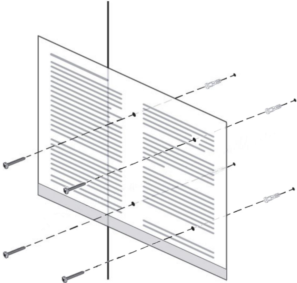
**STEP 2 |** Use a #1 Phillips-head screwdriver to install the appropriate screws into each of the four marked locations:
