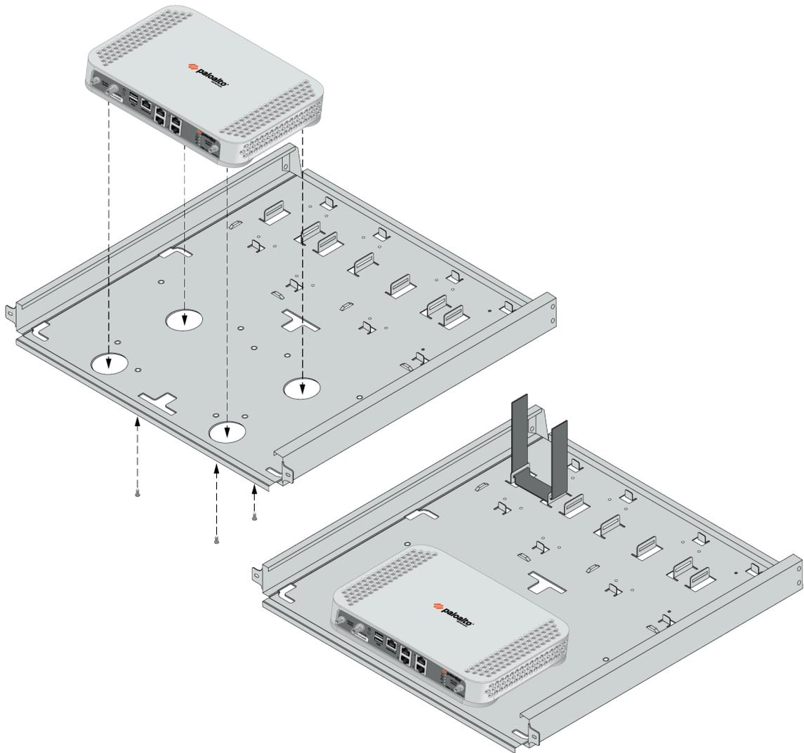
**STEP 5 |** Secure the device in place using three of the provided #6-32 x 3/16" Long Flathead screws.
