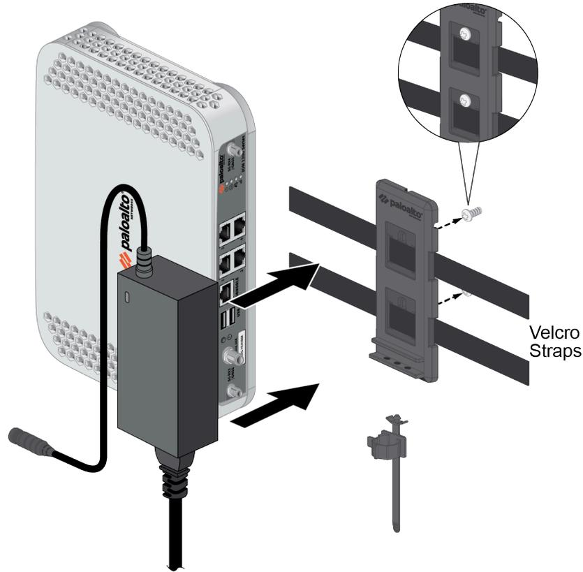
The following image shows a completed installation for an ION 1200 with a single power adapter.
